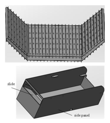
Fig. 3. Top-immersion conveyor belt, bottom-cleaning box
