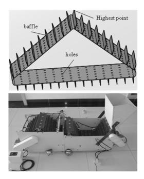
Fig. 5. Top-cleaning conveyor belt, right-actual structure of the prototype
